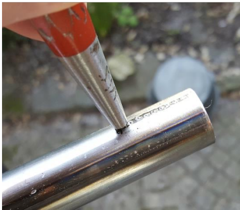
Use the center-punch tool to punch indents along the line, to prevent the drill from walking.
