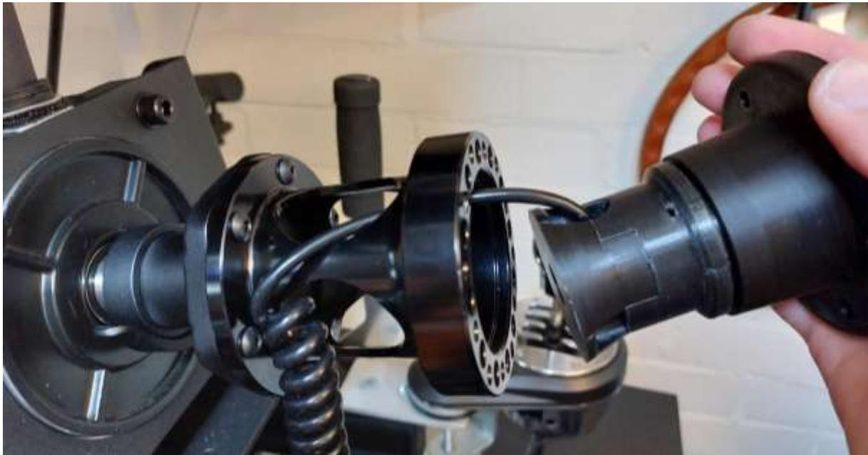
Mount the quick release onto the spacer. Make sure you are using the correct bolt holes in the spacer: only one pattern fits.
