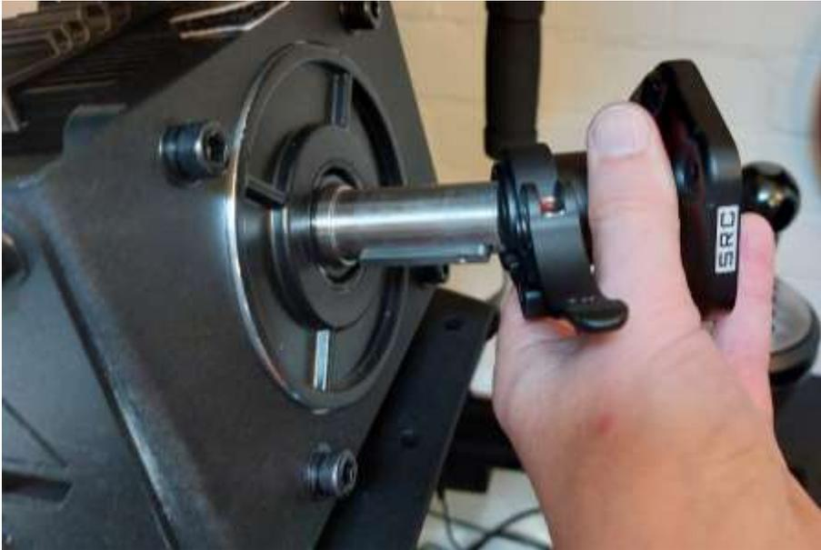
Mount the spacer onto the SRC quick release.
