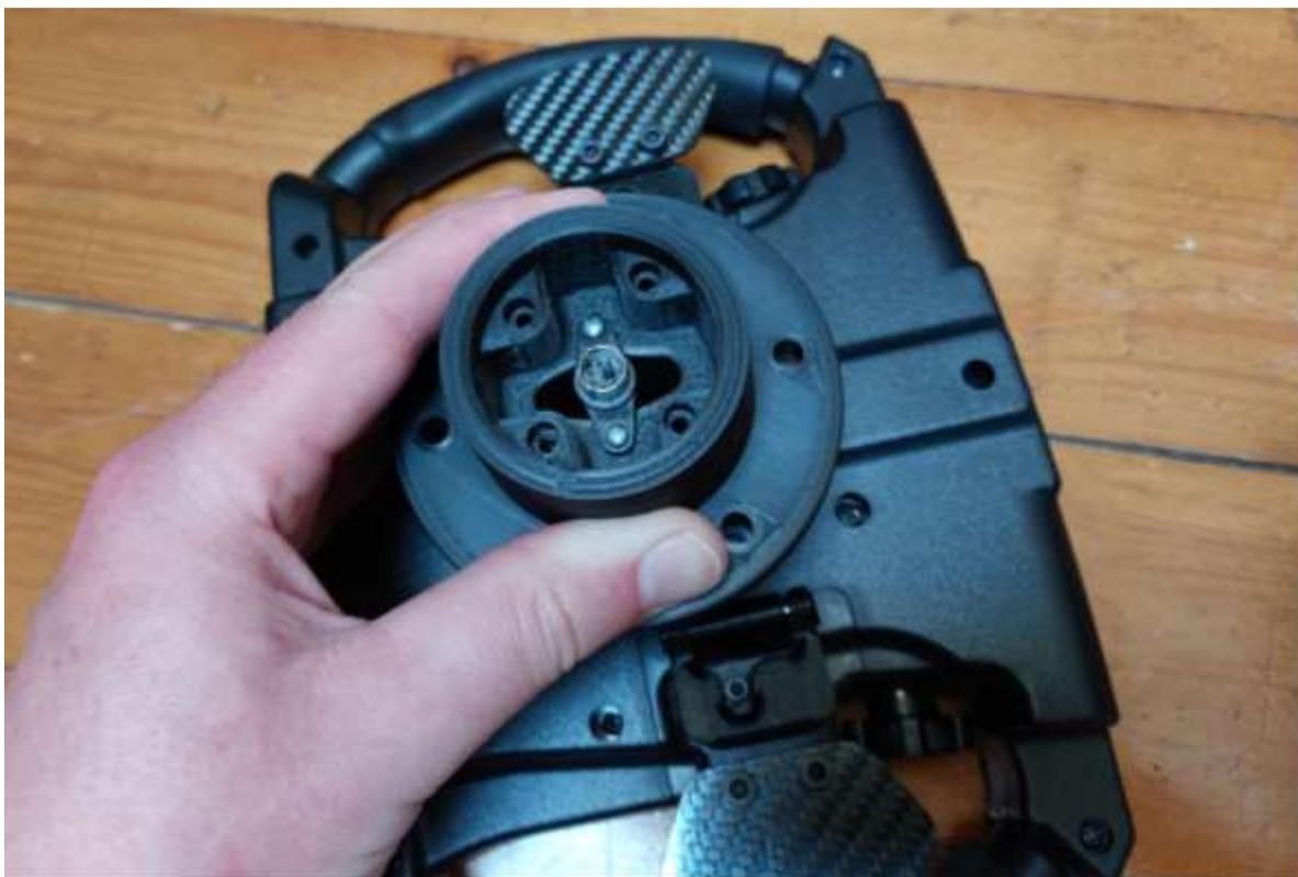
Note: there are 4 holes in this adapter for bolts and nuts to protect against delamination, but I don't think it is necessary (I left the bolts out).
