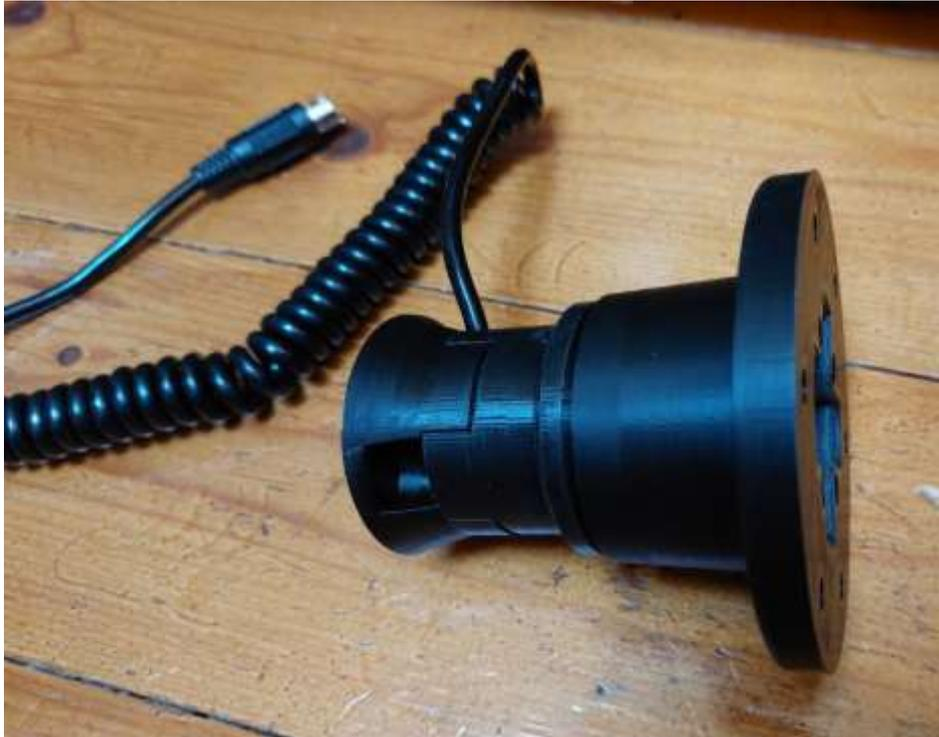
Guide the cable through a hole in the spacer and insert the assembly into the spacer:
