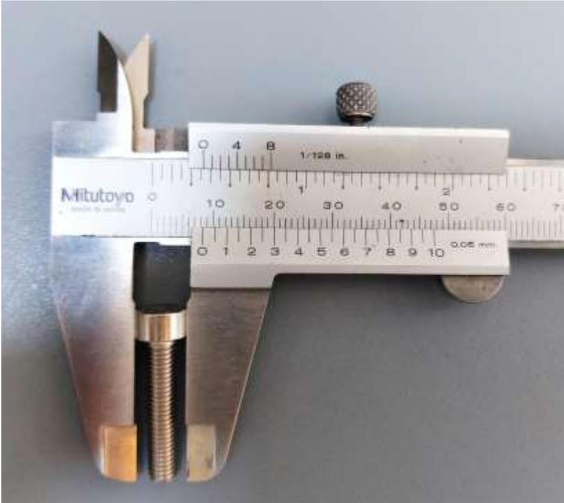
We need to grind the bolt heads down to 7.2 mm. The easiest way to do this is to put two nuts onto the bolt:
