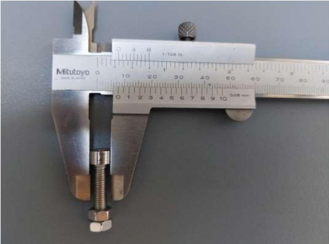
When the size is OK, put the bolt aside to cool down. Mount new nuts onto the next bolt and repeat for all 6 bolts.
