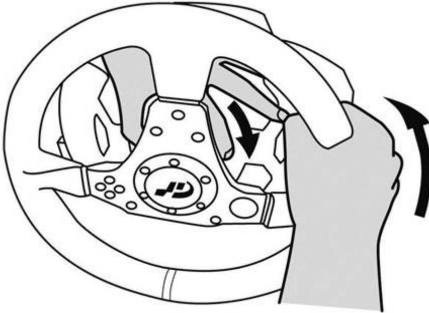
Only after making sure that the central attachment ring is tight, also tighten the small holding screw (taking care not to force or over-tighten the screw).
